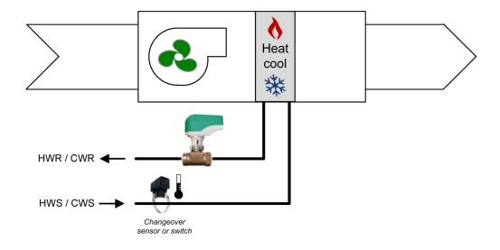
The 2 pipe system consists of a single water coil connected to two pipes (supply and return) and one valvle that can serve as either chill water coil or hot water coil depending on the mode of the system. This type of fan coil cannot cool and heat at the same time and is dependent of the actual mode of the building.
