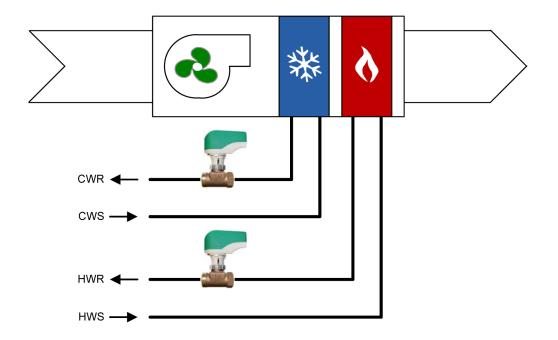
The 4 pipe system consists of two separate cooling and heating water coils. Each coil has its own dedicated set of pipes (supply and return) and valve. This type of fan coil can cool and heat at the same time and is not dependant of the actual mode of the building.
